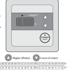
**Notice:** Only commercial model water heaters can achieve temperatures up to 180°F (82°C).
