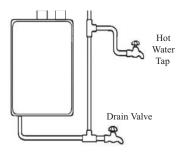
This appliance is not intended for space heating application. Do not connect this heater to waterlines previously used for space heating or non-potable water distribution. All water piping and components shall be suitable for potable water.
