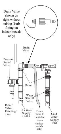
**Notice**: The above illustrates a pressure-only relief valve. If local codes require a combination temperature and pressure relief valve be installed, an extension piece may be needed to ensure that the valve probe is not directly in the flow path of the water.
