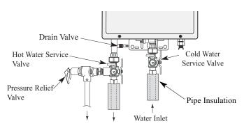
For increased energy efficiency, use pipe insulation. Please install the insulation according to the diagram above, making sure to insulate all the way to the top. **Do not** cover any drain or pressure relief valve(s).
