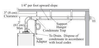
Example B: Typical Horizontal Termination w/ 1/4" per foot <u>UPWARD</u> Slope
