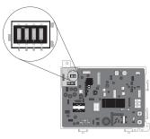
Location of DIP Switches on PC Board.
