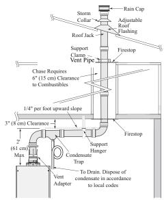
Alternate Vertical Vent Termination with Rain Cap
