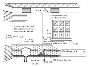
AWARNING: Moisture in the flue gas will condense as it leaves the vent terminal. In cold weather this condensate can freeze on the exterior wall, under the eaves and on surrounding objects. Some discoloration on the exterior of the building is to be expected. However, improper location or installation can result in severe damage to the structure or exterior finish of the building.
