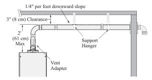
Example A: Typical Horizontal Termination w/ 1/4" per foot <u>DOWNWARD</u> Slope
