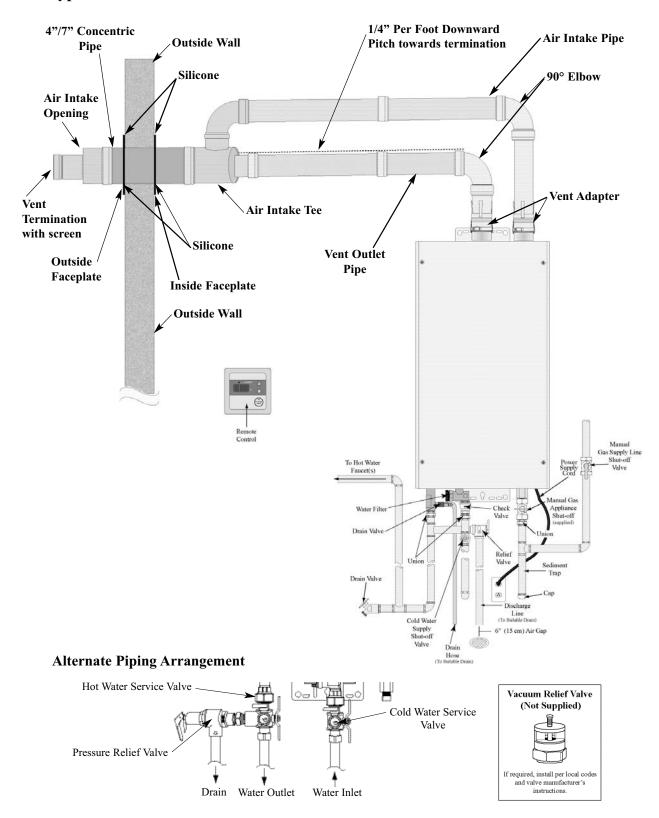
**Typical Installation of Direct Vent Water Heater**
