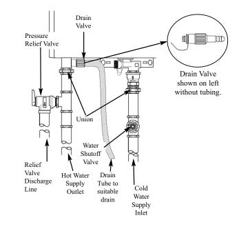
**Notice:** The Figure on the right shows a pressure only relief valve. If local codes require a combination temperature and pressure relief valve be installed, an extension piece may be needed to ensure the valve probe is not directly in the flow path of the water. A WARNING: Do not attempt to convert this water heater for use with a different type of gas other than the type shown on the rating plate. Such conversion could result in hazardous operating conditions.
