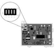
Location of DIP Switches on PC Board.
