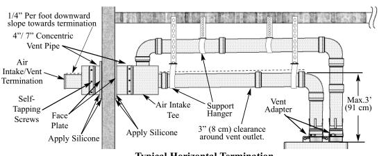
Typical Horizontal Termination w/ ¼" per foot DOWNWARD Slope towards termination
